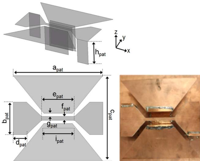
Fig. 17. Geometry and design parameters of the proposed pattern diversity antenna.
