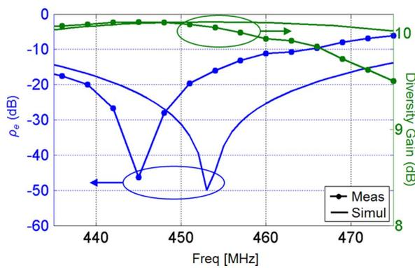
Fig. 21. Envelope correlation ( $\rho_e$ ) between radiation patterns of two antenna elements in the proposed pattern diversity antenna and its diversity gain.
