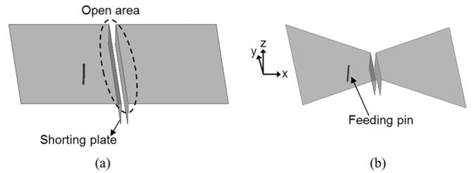
Fig. 1. (a) Proposed microstrip antenna with an open area in its middle and (b) bow-tie version of the proposed microstrip antenna over an infinite ground plane.
