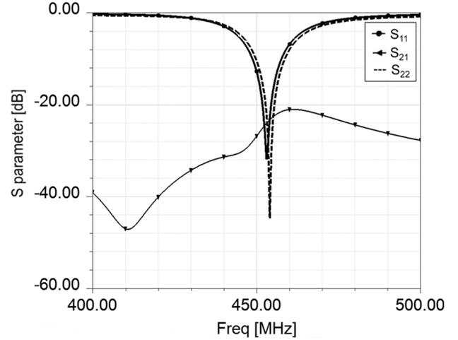
Fig. 10. Simulated  $S_{11}$ ,  $S_{21}$  and  $S_{22}$  of the proposed polarization diversity antenna.
