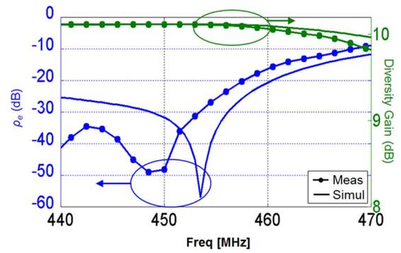
Fig. 14. Envelope correlation ( $\rho_e$ ) between the two common aperture antenna elements in the proposed polarization diversity antenna and its diversity gain.
