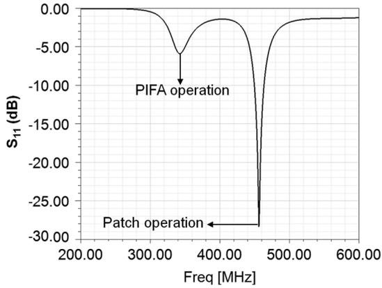
Fig. 4. Simulated  $S_{11}$  of the proposed bow-tie microstrip antenna shown in Fig. 3.
