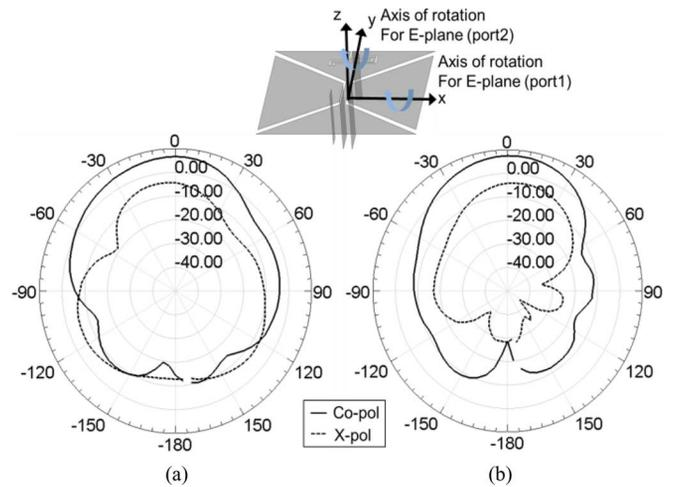
Fig. 15. Measured radiation patterns (gain) on E-planes of two bow-tie microstrip antennas: (a) Port1: ON and Port2: OFF ( $50 \Omega$  terminated) and (b) Port1: OFF ( $50 \Omega$  terminated) and Port2: ON.
