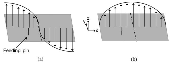
Fig. 2. Distributions of (a) voltage and (b) current on the  $\lambda_g/2$  microstrip antenna with x-polarized radiation over an infinite ground plane.
