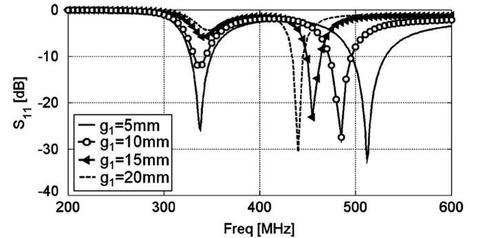
Fig. 7. Simulated  $S_{11}$  of the proposed bow-tie microstrip antenna versus  $g_1$ .
