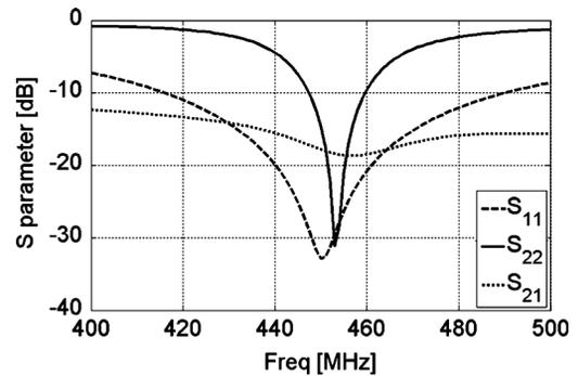
Fig. 18. Simulated  $S_{11}$ ,  $S_{21}$  and  $S_{22}$  of the proposed pattern diversity antenna.
