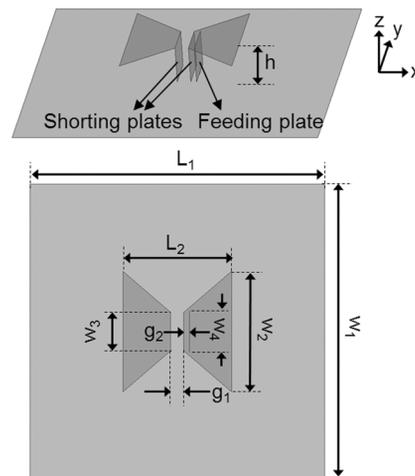
Fig. 3. Geometry and design parameters of the small-size bow-tie version of the proposed microstrip antenna with an open area at its waist.
