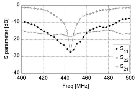
Fig. 19. The measured  $S_{11}$ ,  $S_{21}$  and  $S_{22}$  of the proposed pattern diversity antenna.
