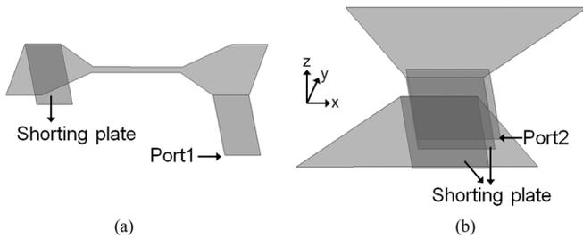
Fig. 16. (a) Folded monopole antenna with omnidirectional radiation pattern and (b) proposed bowtie microstrip antenna with broadside radiation pattern.
