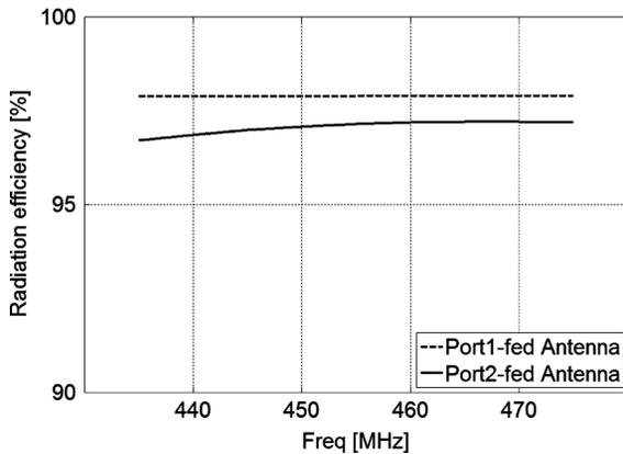
Fig. 20. Simulated radiation efficiency of two antenna elements in the proposed pattern diversity antenna.
