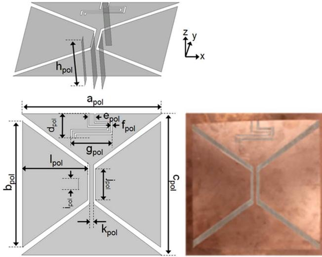
Fig. 9. Geometry and design parameters of the proposed polarization diversity antenna.
