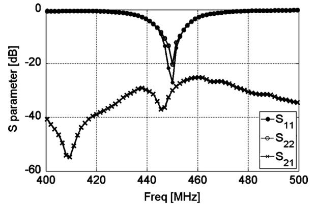
Fig. 11. Measured  $S_{11}$ ,  $S_{21}$  and  $S_{22}$  of the proposed polarization diversity antenna.
