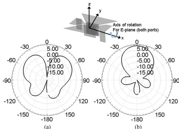
Fig. 22. Measured radiation patterns (gain) on E-planes of the folded monopole antenna and proposed bow-tie microstrip antenna: (a) Port1: ON and Port2: OFF ( $50 \Omega$  terminated) and (b) Port1: OFF ( $50 \Omega$  terminated) and Port2: ON.
