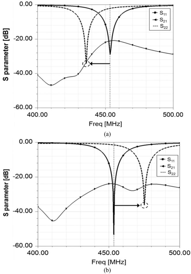
Fig. 12. Simulated  $S_{11}$ ,  $S_{21}$  and  $S_{22}$  of the proposed polarization diversity antenna with 5 mm (a) increased or (b) decreased  $l_{pol}$ .
