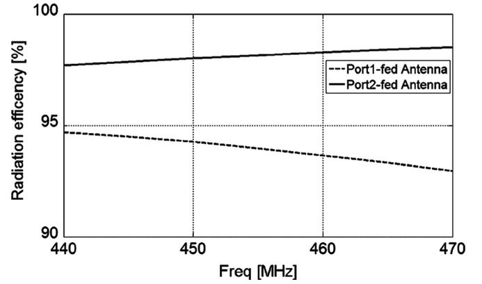
Fig. 13. Simulated radiation efficiency of two antenna elements in the proposed polarization diversity antenna.
