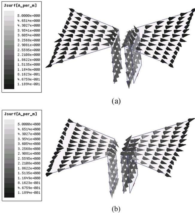
Fig. 5. Current distributions of the proposed antenna in Fig. 3 at (a) 342 MHz (PIFA mode) and (b) 456 MHz (patch mode).
