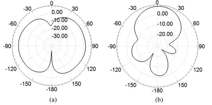
Fig. 6. Simulated radiation patterns (gain) of the proposed bow-tie microstrip antenna on E-plane (xz-plane) at two resonant frequencies, corresponding to (a) PIFA mode and (b) patch mode. Antenna geometry is shown in Fig. 4.
