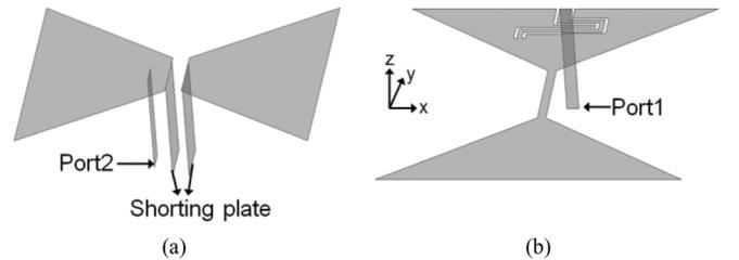
Fig. 8. (a) Proposed bow-tie microstrip antenna with x-pol and (b) conventional bow-tie microstrip antenna with y-pol.
