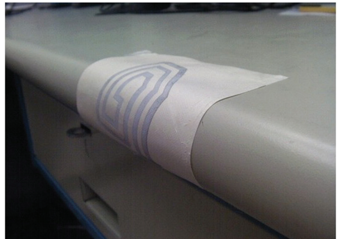
Figure 14b. A demonstration of the nanopaper antenna's flexibility.
