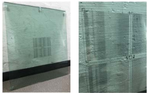
Fig. 16. Laminated glass with the PET film of Fig. 15 inserted.
