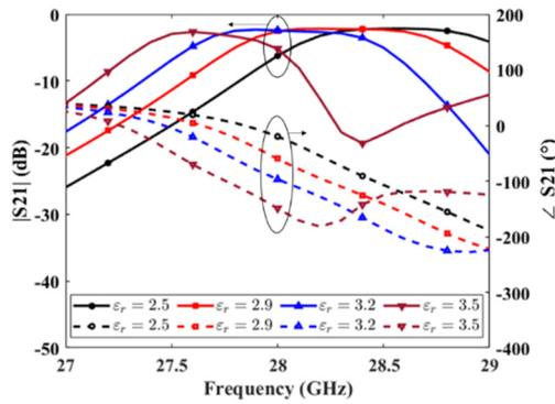
Fig. 6. Frequency responses of the unit cell regarding the LC permittivity.
