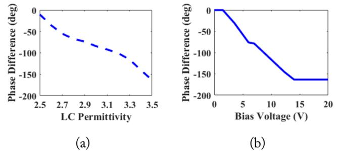
Fig. 10. Simulated and measured results of phase differences of the LCTA unit cell (Sim: at  $28 \text{ GHz}$ , Meas: at  $28.5 \text{ GHz}$ ).
