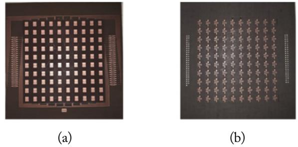
Fig. 8. A photograph of the fabricated sample: (a) dipole layer with bias lines, and (b) meander layer.
