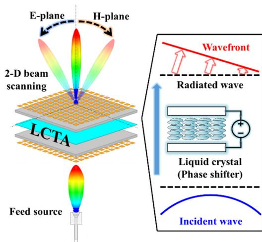
Fig. 1. Operation principle of an LCTA. The LCTA compensates for a phase of an incident wavefront from the feed source.
