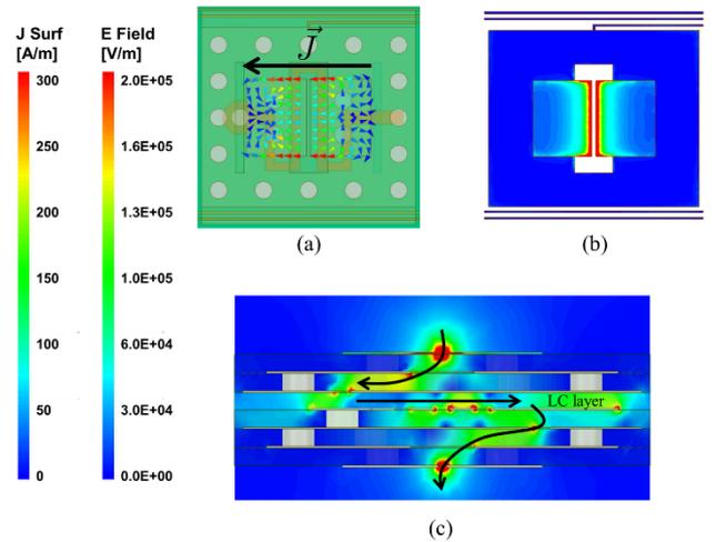
Fig. 5. Field distribution of the proposed unit cell design: (a) top view (current vector), (b) top view (E-field on dipole and bias layer), and (c) unit cell cross-section on E-plane (E-field).
