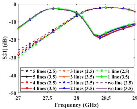
Fig. 7. Frequency responses of the unit cell regarding the number of bias lines. Numbers inside the brackets refer to the LC permittivity.
