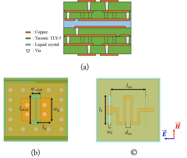
Fig. 4. Geometry of the unit cell: (a) unit cell cross-section on E-plane (black dash: via wall), (b) dipole layer, and (c) stripline layer;  $w_p=1.8$ ,  $l_p=1.4$ ,  $w_{slot}=0.9$ ,  $l_{slot}=2.6$ ,  $w_t=0.2$ ,  $l_t=2.6$ ,  $d_m=0.4$ , and  $l_m=3.0$  (unit: mm).
