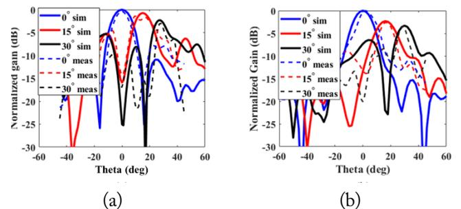
Fig. 11. Simulated and measured radiation pattern results on (a) E-plane and (b) H-plane (Sim: at  $28 \text{ GHz}$ , Meas: at  $28.5 \text{ GHz}$ ).
