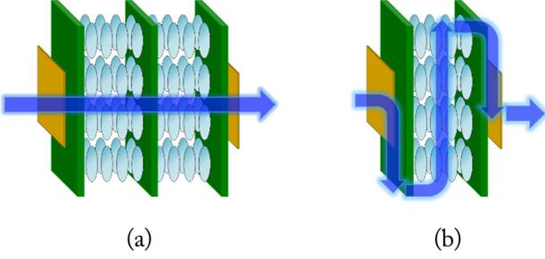
Fig. 2. Examples of ways to expand the phase tuning range: (a) increasing LC thickness (conventional) and (b) converting transmission path (proposed).
