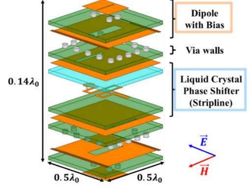
Fig. 3. Exploded view of the proposed unit cell design.
